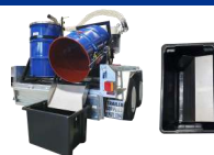
Drum waste discharge chute with bucket
